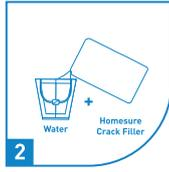
Add HomeSure Crack Filler in water to create a paste.
