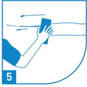
Apply mixture to fill the entire depth of the open crack using a steel trowel / blade.
