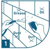
The substrate needs to be cleaned and made free from grease and loose particles. Then dampen the surface with clean water.
