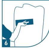
6 Pre wet the 1<sup>st</sup> coat need based and then apply 2<sup>nd</sup> coat.
