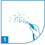
Dampen the opened crack up to 4mm thick & allow excess water to drain.
