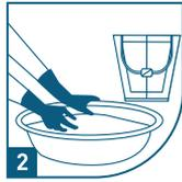
Add Ready Mix Plaster to potable water & mix well for 5-10 mins. (Recommended mix 15-17% water)
