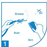
1 Clean the surface with sand paper / putty blade & then dampen the surface.
