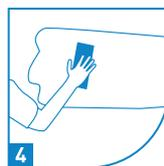
4 Apply 1<sup>st</sup> coat with putty blade. (Thickness of 0.5-1 mm)
