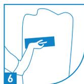
6 Apply 2nd coat & allow the surface to dry completely. (Thickness of 0.5 - 1mm.)
