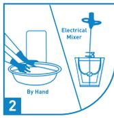
2 Add Putty in water to obtain a lump free paste & mix well. (Recommended mix 40% water)
