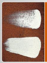
Photo compares one brush stroke of quality primer (top), with one stroke of the same primer mixed with OWATROL® OIL.
